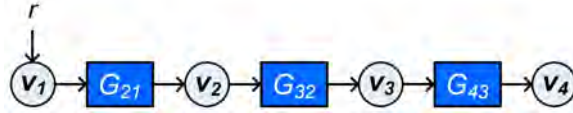
Figure 1.6: Vehicle-based dynamic network representation as described in [94]. G_{ij} represents the dynamics (transfer function) from the j^{\text{th}} vehicle velocity to the i^{\text{th}} vehicle velocity. The variables v_i represent the velocity of the i^{\text{th}} vehicle. The variable r refers to the excitation given to the leading vehicle, the velocity profile.
