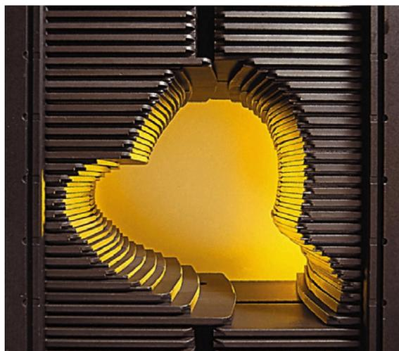
**Figure 1.2:** Example of a multileaf collimator. Image courtesy of Varian Medical Systems, Inc. All rights reserved. Source: <https://bit.ly/3FA0B56>
