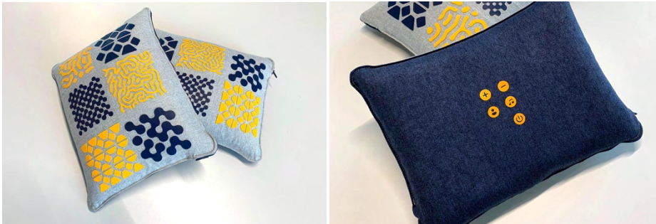
Figure 5.1. Vita served as an example of audio-based technology: (left) Vita is a cushion with conductive touchpads to play audio content and (right) with buttons on the reverse side to adjust the settings or volume.
