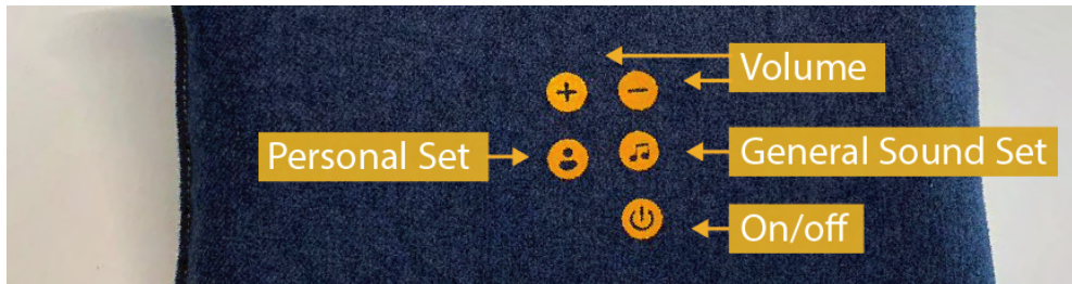
Figure 6.2. The personal and general sound sets can be selected by pressing the buttons on the reverse side of Vita to go through the sets, with voice feedback indicating which set is selected.
