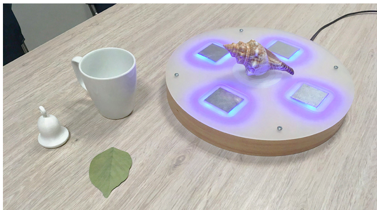
Figure 2.1. Placing the everyday object (e.g. seashell) on the Dementia Soundboard triggered the corresponding soundscape (e.g. beach). By touching the surrounding touchpads, each layer (e.g. beach_children) could be activated or deactivated.
