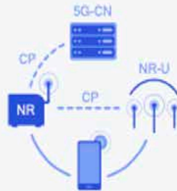
Scenario B Carrier aggregation NR with 5G-CN 2 and NR-U
