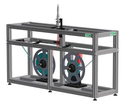
of pieces of composite tape pasted on paper carrier tape, which can improve the productivity and accuracy of the existing systems. The new tape requires modifications in the current pre-heating system to avoid burning or heating of the carrier tape. Also, the newly developed pre-heating system needs to be experimentally verified by developing a test setup.
