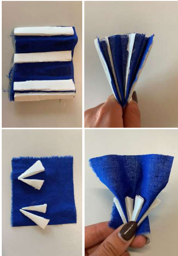
Figure M. Foam glued to fabric to test different origami structures for folding the fabric.
