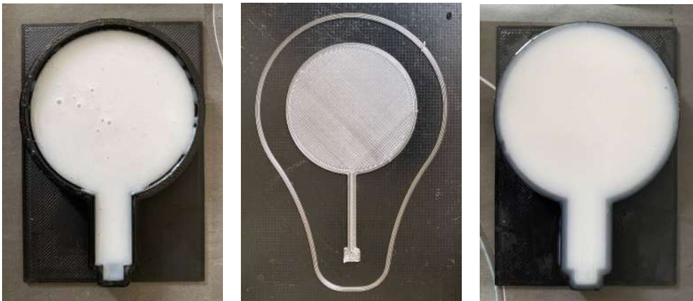
Figure L. On the left the silicone filled to half of the mold. In the middle the separator made of PVA filament. On the right the mold with separator is completely filled.
