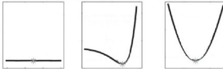
Figure 5.1: Three plots of J(\theta) for a one-dimensional parameter space are depicted regarding three different cases of identifiability. On the left a structural non-identifiable parameter, in the middle a practical non-identifiable parameter and on the right an identifiable parameter. Adapted from: ‘Structural and practical identifiability analysis of partially observed dynamical models by exploiting the profile likelihood.’ by A. Raue et al, 2009, Bioinformatics , 25, 1923–1929 [62].
