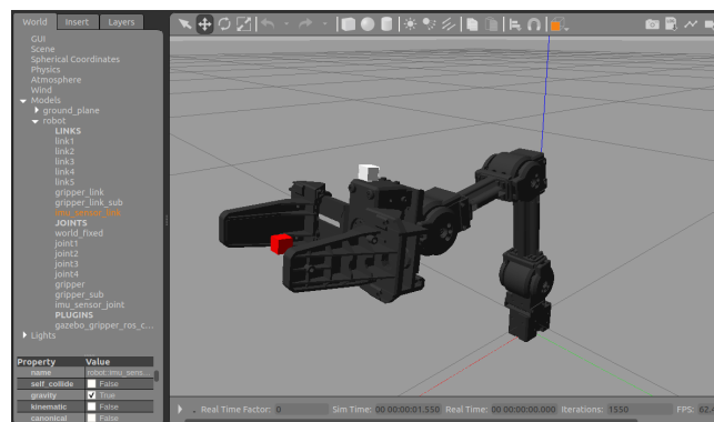
Figure 4.8: IMU sensor attached to the manipulator
