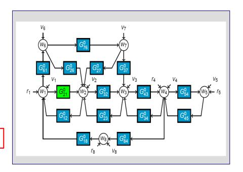
• Identify a local (set of) module(s) from a (sub)set of measured  $r_k$  and  $w_\ell$
