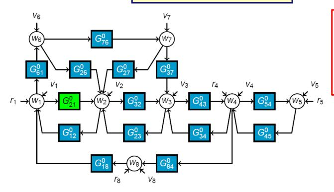
To maintain  $G_{ji}^0$  these should be "blocked" by measured nodes (predictor inputs)
