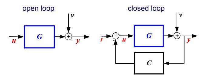
Identify a plant model  $\hat{G}$  on the basis of measured signals u, y (and possibly r)
