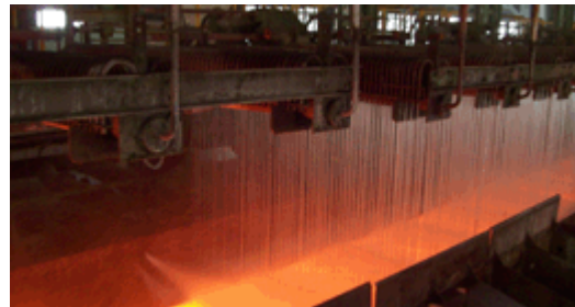
Figure 1: Hot strip mill cooling system using water jets
