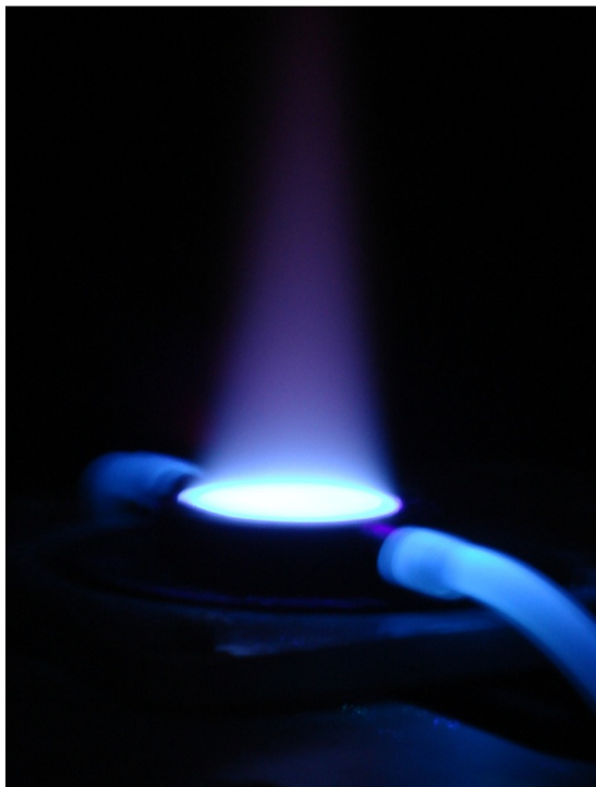
Picture: A ZnO:Zn phosphor coated plate when excited by 355 nm YAG laser in presence of a methane/air flame.
