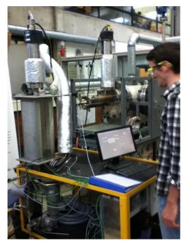
In a lab of the TU/e an experimental set-up of the once-through steam generator (15kW thermal power) was realized. Also a finite volume model of the once-through steam generator was developed.
