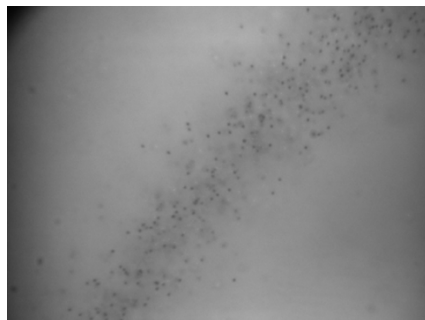
Figure 1: An optical microscope image showing beads being driven by passive micro-pump
