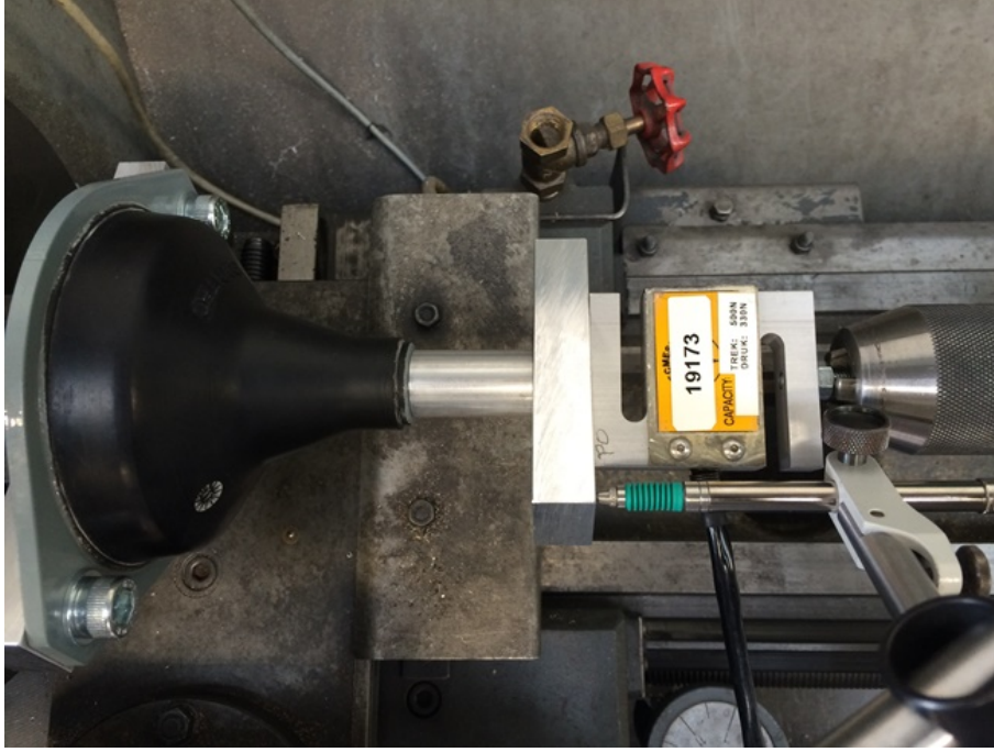
Figure D.2: Detailed overview isolator and sensors quasi-static setup, detailed.
