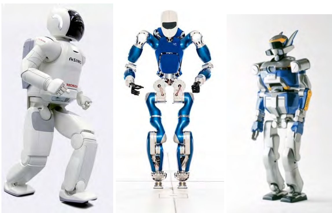
(a) The ASIMO humanoid robot. Image courtesy Honda 1 . (b) The TORO humanoid robot. Image courtesy DLR 2 . (c) The HRP-2 humanoid robot. Image courtesy kawada 3 .
