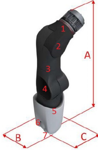
Figure 3.1: ULNA joint numbers and general dimensions A = 620\text{mm} , B = 150\text{ mm} and C = 280
