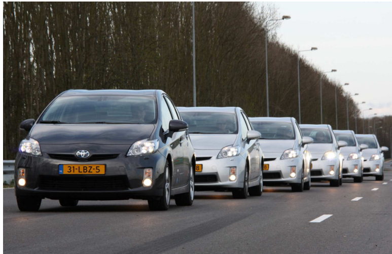
Figure 1.1: Platoon of CACC-equipped vehicles [7]
