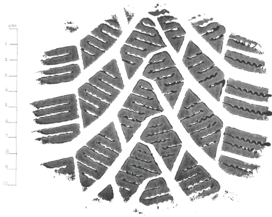
Figure 5.10: Tyre 3 contact patch at Inflation pressure: 240 kPa and Vertical force: 3500 N
