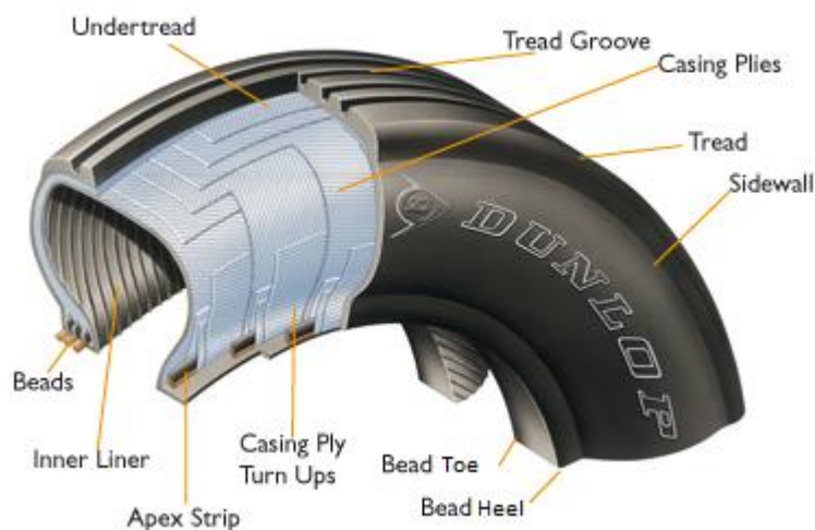
Figure 2.1: Cross-section of the Bias tire type [32].
