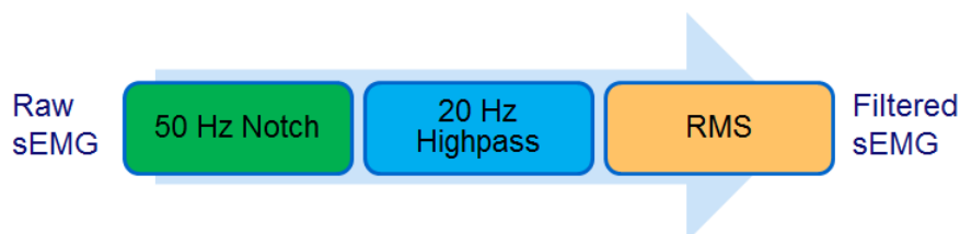
Figure 2.2: The sEMG signal processing.
