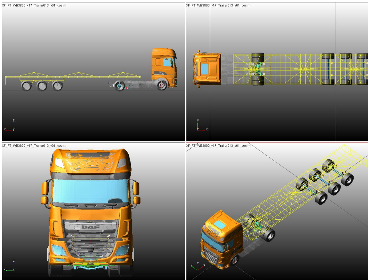
Figure 29. ADAMS vehicle model used for vehicle simulations.
