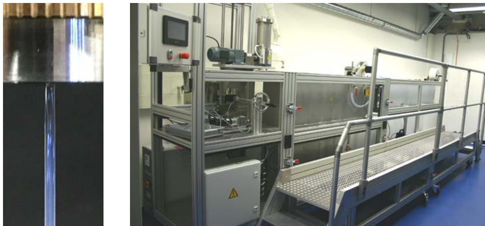
The nascent fiber leaving the spinneret and the spinline.
