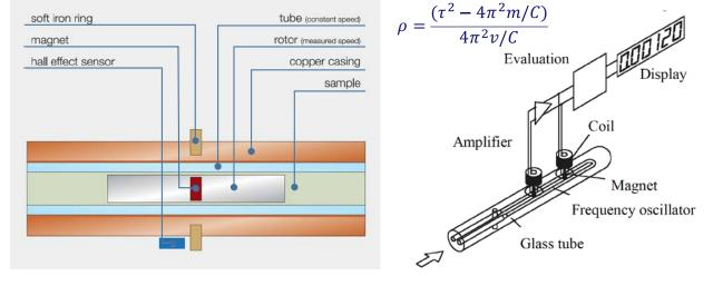
Principle of rotational viscosity meter and oscillating U-tube density measurement. (C = spring constant)
