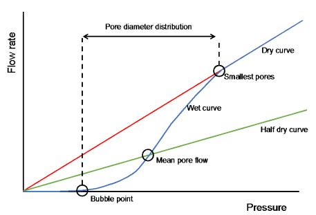
The results of porometry measurement.
