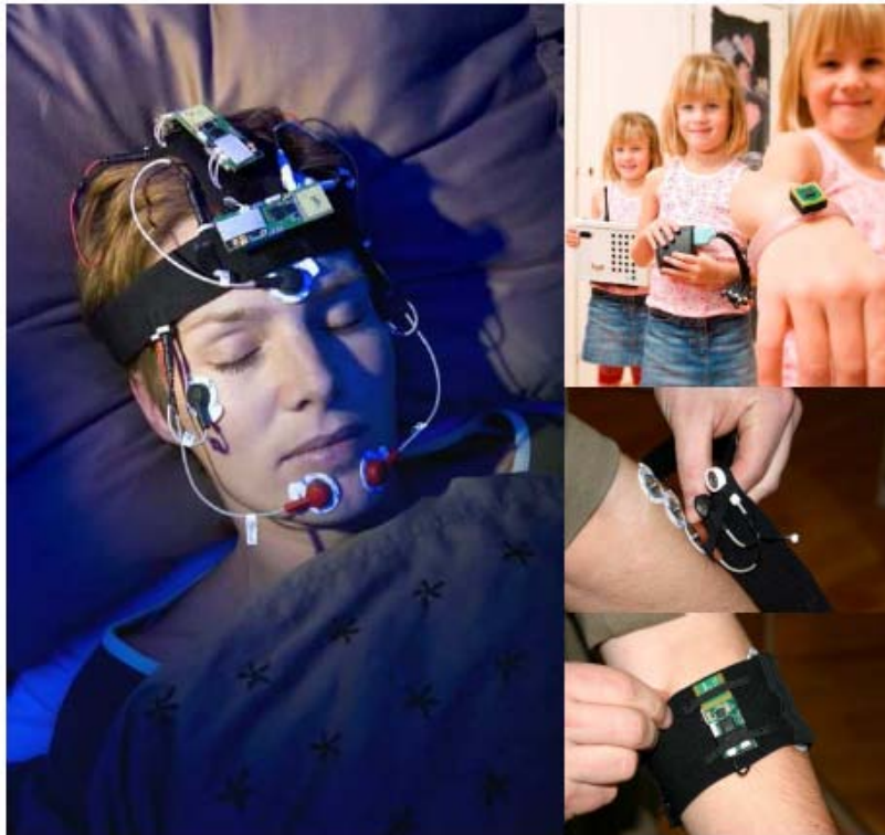
Wireless EEG, ECG, EMG and EOG monitoring
