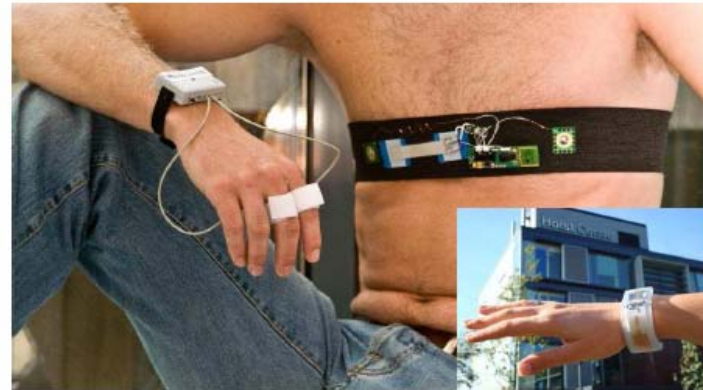
Wireless ECG, respiration, Skin Temperature and Skin conductance monitoring
