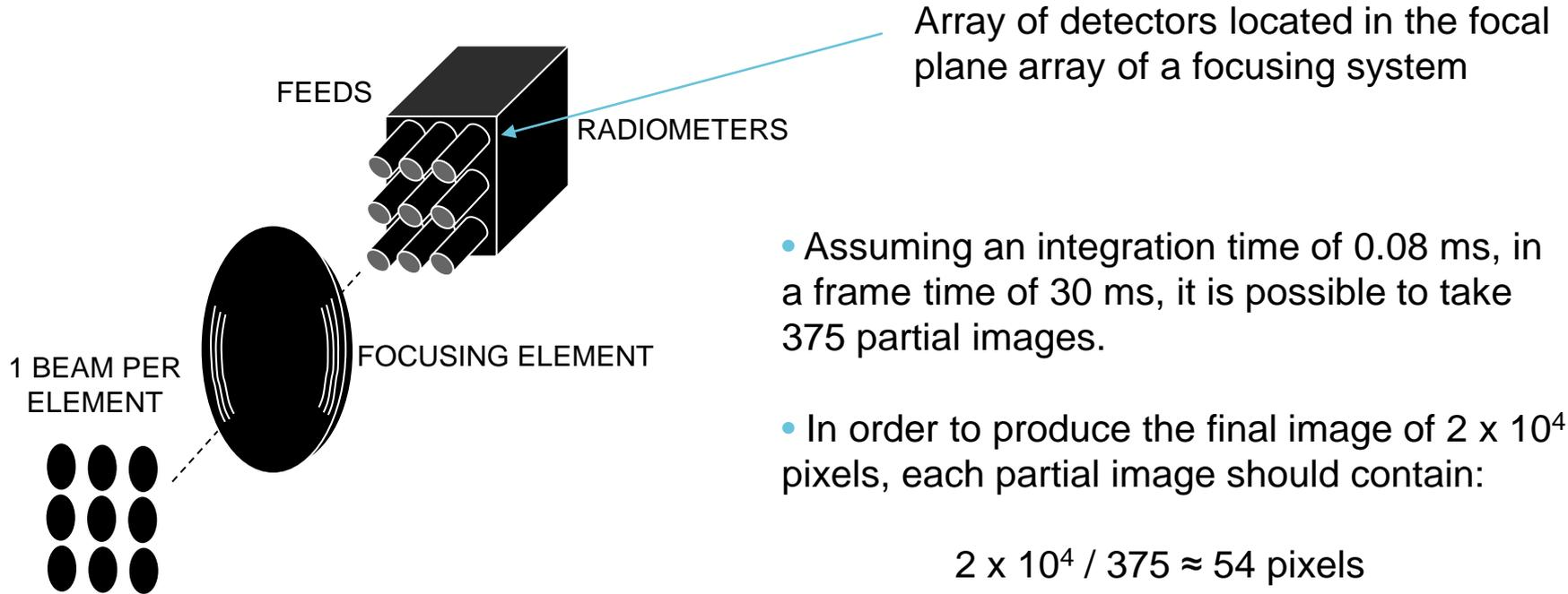
A focal plan array of 54 elements would be able to produce a real time image.
