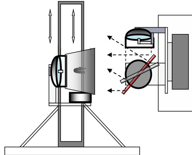
Antenna scanned vertically + rotating mirror for horizontal scanning
