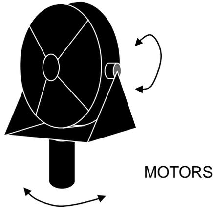
Antenna scanned in two dimensional plane
