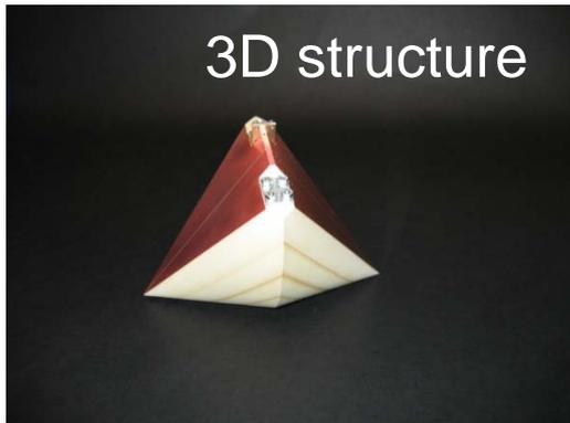
Original Ultra-wide-band leaky lens antenna (TNO-ESA patent)
