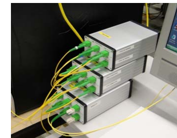
Cascaded Add & Drop filters
