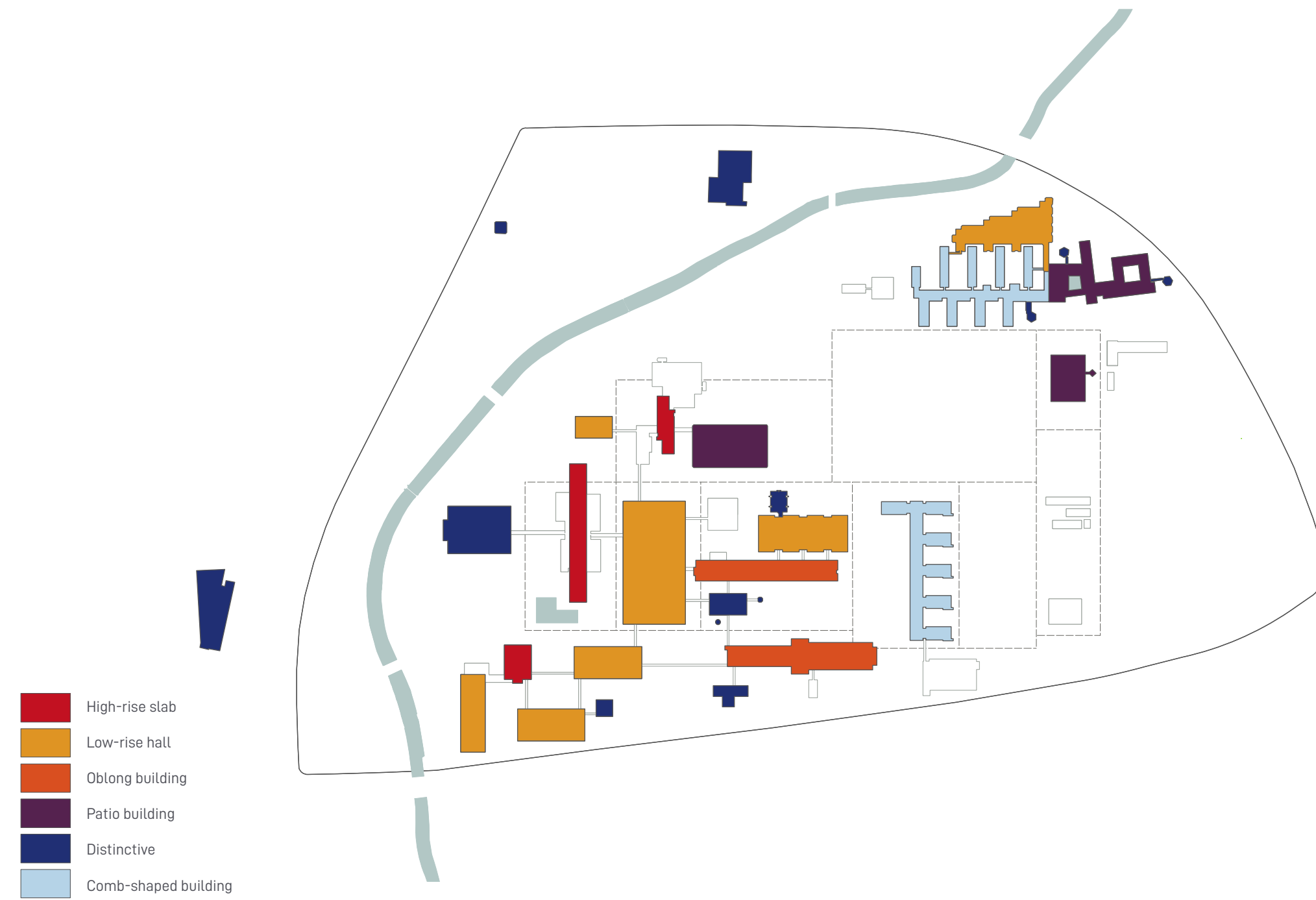
Fig. 2.10 — The building types (main volumes) applied in the first and second building rounds; the 'comb-shaped building' will disappear later as it occupies too much space
