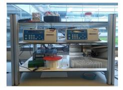
In order to accelerate the screening of the continuous-flow photoreaction and development of new photocatalytic reactions, a fully automated platform, containing reagent storage, selection, pumping, mixing, reaction, analysis and sample collection, is being established. This platform is still in the development phase and some control codes need to be programmed and optimized.
