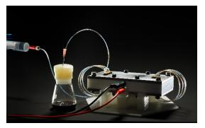
In our group, an electrochemical microreactor is used to conduct aziridation reaction in continous-flow mode. Performing reaction in flow enables to overcome mass-transfer limitation and provides equal charge distribution over the whole reaction mixture increasing productivity and selectivity of the transformation.
