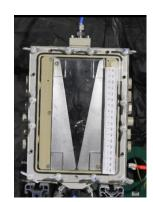
This research will mainly focused on plasma assisted nitrogen fixation process. Based on existing gliding arc plasma discharge reactor, investigation on NOx production from atmospheric air will be conducted.
