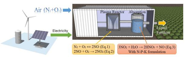
The aim of this research is to increase the energy efficiency for nitrogen fixation and increase the productivity of the plasma assisted fertilizer production process. The liquid fertilizer produced will be applied to meet the demand of real case cultivation, including soil growing and hydroponics.
