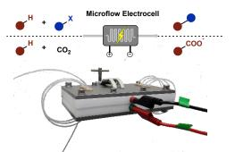
In our group an electrochemical microreactor was recently designed. With this reactor new electrochemical methodologies were explored. At the moment, investigation of electrochemical C—H activation reaction and  $CO_2$  activation for organic chemistry methodologies are under development.
