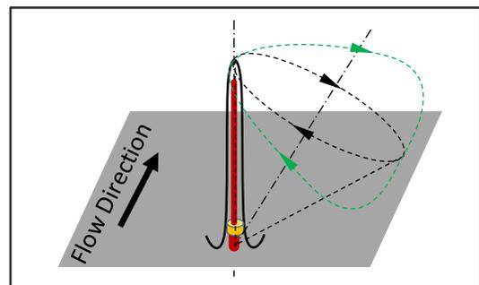
Figure 3: Example of two different paths traced by the cilia actuated by magnets of different shapes. One profile may generate better flow than the other one.
