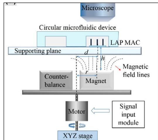
Figure 2: Magnetic actuation system with placement of fabricated cilia in a microfluidic device and magnet position parameters indicated<sup>2</sup>.
