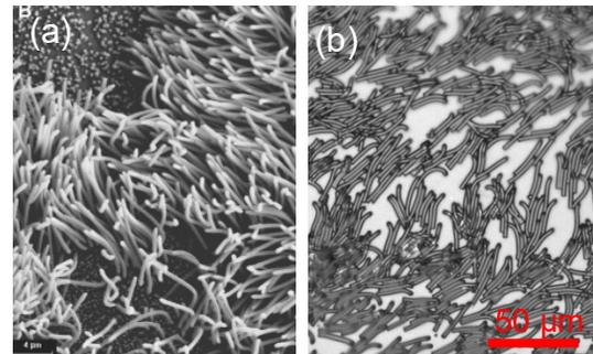
Figure 1: (a) Cilia present in the human Fallopian tubes<sup>1</sup>. (b) Cilia fabricated in the Microfab lab.
