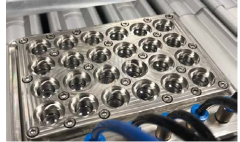
Figure 1: heart on chip platform. A PDMS film is at the bottom of each well, performing sinusoidal up and down movement.
