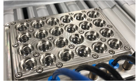
Figure 1: 'heart on chip' platform. A PDMS film is at the bottom of each well, performing sinusoidal up and down movement. Cylinders for pneumatic actuation can be seen underneath the chip.
