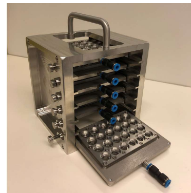
Figure 2: high-throughput system with 144 wells.
