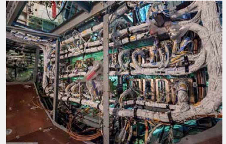
Airbus 380-800: 470 km of wire, weighing 5700 kg
