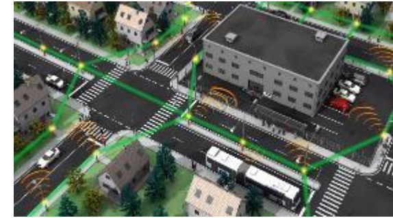
Safe crossing application based on JCAS
