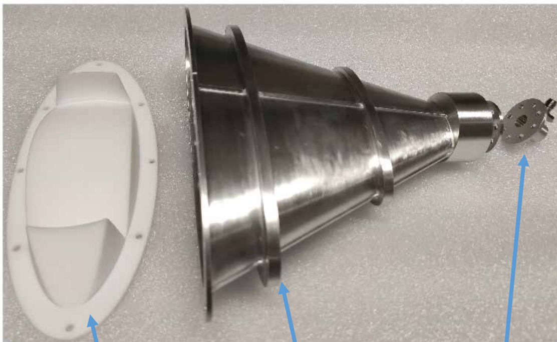
Dual polarized lens-horn antenna n257 band (26.5-29.5 GHz)
