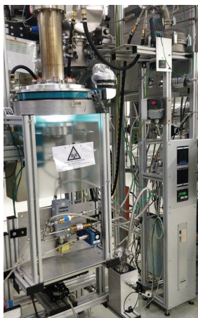
Figure 1. Left: Reactive zone of the microwave plasma reactor at the University Duisburg-Essen. Right: Few-layer graphene as seen under the transmission electron microscopy.
