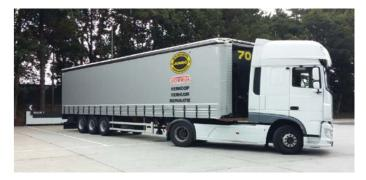
To test the designed system it was implemented on a DAF Euro VI truck, making use of dSPACE Rapid Control Prototyping (RCP) hardware and software. Additionally, a dummy dock was constructed, where the necessary dock-side components of the system could be mounted. After implementation and testing, the designed architecture and control concept have proven successful in parking the truck autonomously
