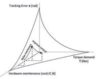
which degrades machine cost and effectiveness. Relaxing mechanics, i.e. reducing stiffness and increasing gap size, can remedy this, but degrades tracking performance due to the resulting side effects: torsional vibration and backlash. Torsional vibration and backlash compensation using non-linear feedforward control, is therefore applied to recover performance.
