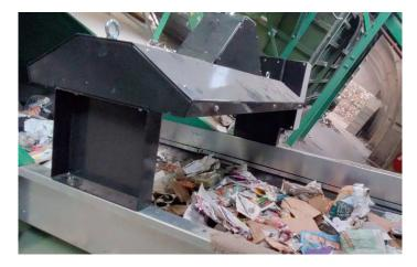
The author, Aneesh Ashok Kumar, was involved in the design and development of such a prototype together with Bollegraaf, using a camera and AI based approach to identify different material classes via object detection, and to estimate the waste-stream composition.
