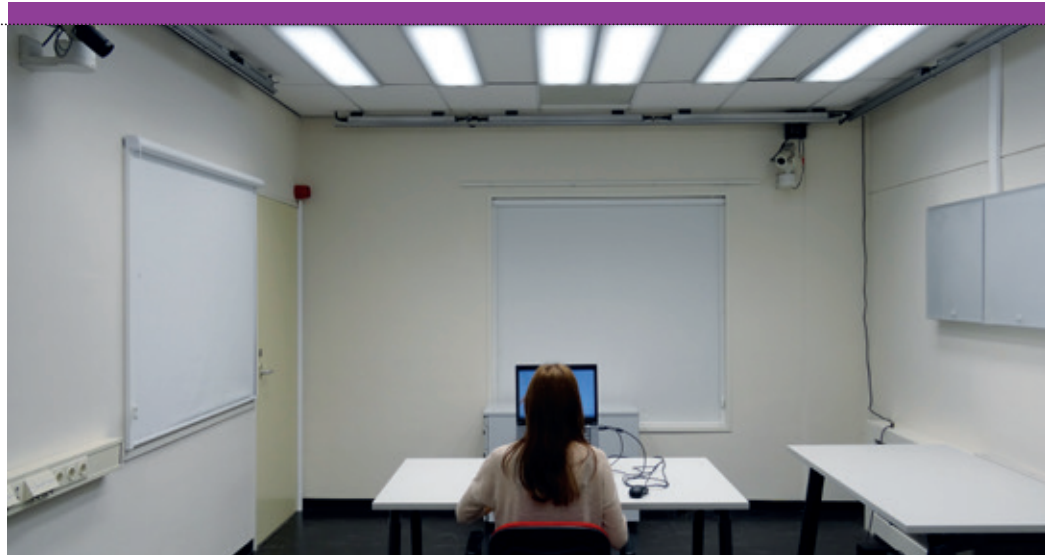
The study was conducted in a simulated office environment at the lighting laboratory of the IPO building. Savio ceiling luminaires were used to create the desired lighting conditions.
