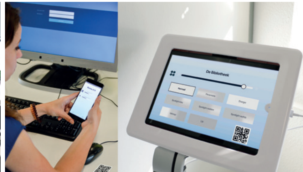
Figure 2. The two user interfaces for lighting control: a smartphone app for lighting control at a desk, and a tablet for lighting control dedicated to meeting rooms.
