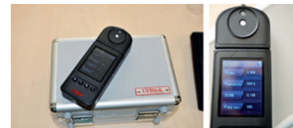
Figure 2: An example of a commercially available product, (UPRTek) which implemented Stroboscopic Visibility Measure (SVM).
