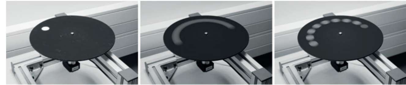
Figure 1: (left) A disk with a black surface and a white spot, (middle) an impression of the appearance of the rotating disk under non-modulated light, giving rise to the perception of a blurred image, and (right) the rotating disk under modulated light, resulting in a visible stroboscopic effect.
