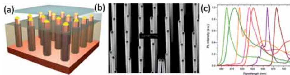
Fig. 1: (a) Schematic of a nanowire LED, (b) electron microscope image of 100 nm diameter nanowires, (c) Observed tuneable emission of GaP-based nanowires.
