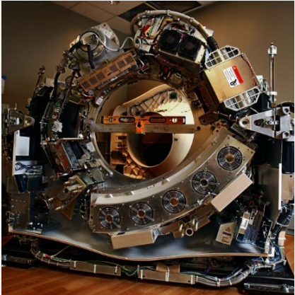
Direct-drive system of CT-scanner
