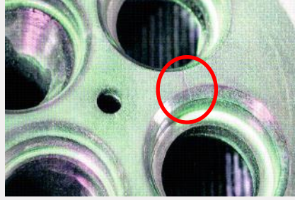
DAF cylinder heads: micro-crack formation
