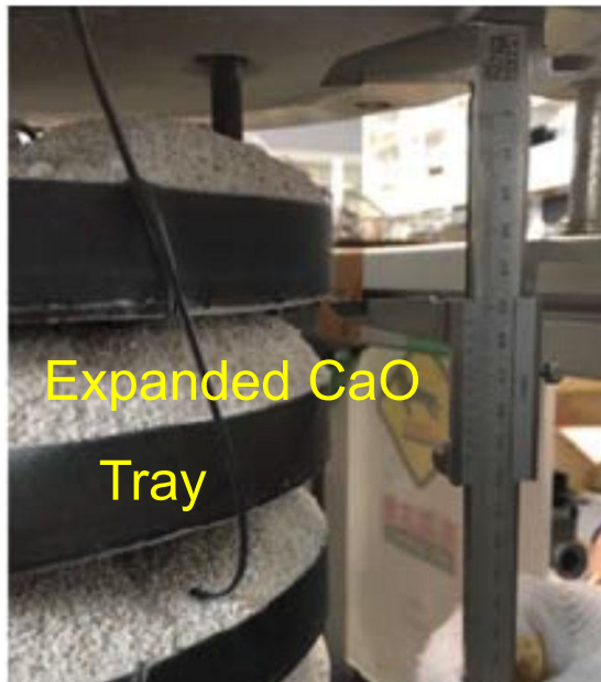
Fig. Overflow of \text{Ca(OH)}_2 material from bed trays after reactions by material expansion.
