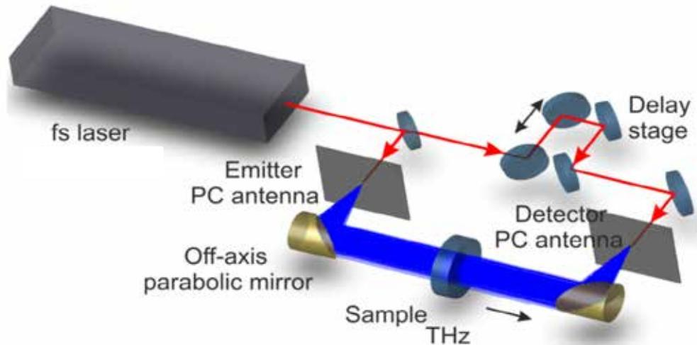
THz time domain spectroscopy is based on ultrashort optical pulses to generate and detect single (or few) cycle THz pulses
